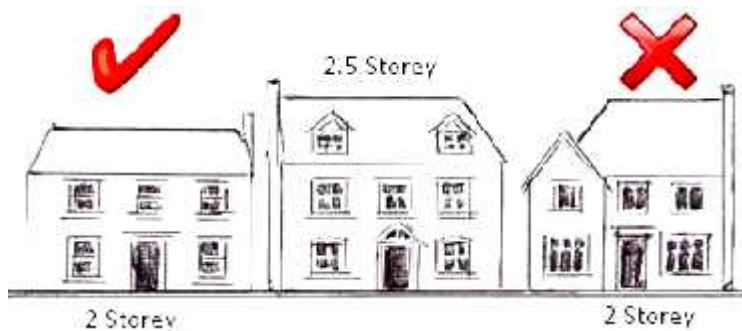
Fig 6.5: Example of Acceptable and unacceptable 2 storey heights
