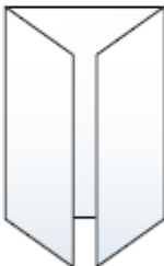
Open gate fold The two parallel folds fold in to meet in the middle without overlapping.
