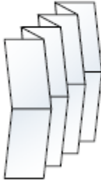
Map fold Paper zig zags like a concertina then folds in the middle.
